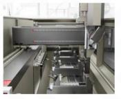
Thanks to its built-in automatic magazine with capacity for 8 tools, GARNET XS4 saves time when switching to different operations.The GARNET XS4, which positions its clamps ful-ly automatically using the X-axis, completely takes on the user's workload
