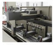
Double-Linear Guide bridge systems have are more rigid and durable compared to single-Linear Guide bridge systems. Reduced vibration and allows for more precise processing of the profiles.
