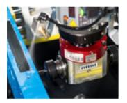
By focusing on providing convenient solutions for customers, and combining power and precision, GARNET XS lets the processing capacity be only limited by the users imagination, thanks to the 5.5 kW spindle motor with automatic tool replacement feature.
