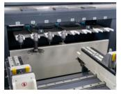
Thanks to its built-in automatic magazine with capacity for 8+1 tools, GARNET XS saves time when switching to different operations.
