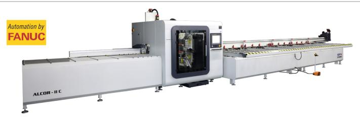
The servo 8-axis CNC profile profile machining and cutting center **ALCOR - II C** has been developed to carry out all-inone cutting, milling, drain channel opening, punching and marking operations on profiles, and to perform special nonstandard operations (punching, channel opening etc.) on different profiles. Thanks to its individually operating units, **ALCOR - II C** has been designed to offer maximum efficiency in less time.
