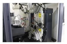
7 units of fan cooled spindle motors that can function and be positioned as different angles enables an unlimited operational capability on 4 surfaces of the profile.
