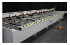
Thanks to the feeding capacity of 10 profiles, the conveyor structure enables batch processing, letting the machine to be used in the most efficient manner.
