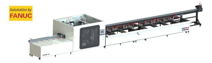
**ALCOR - IV** has been developed to perform cutting, surface treatment and notching operations of wide aluminum and PVC profiles. **ALCOR - IV** is designed to achieve the highest efficiency in the least amount of time with its units that can operate independently of each other.
