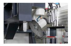
550 mm diameter saw that can cut at any angle between 0° and 180° thanks to its 5-axis movement capability, the saw allows cutting and end-milling operations of profiles up to 300 mm wide.
