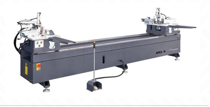
APEX - II, which has automatic hydraulic double head corner crimping, is used for corner binding processes for aluminium profiles. Incorporating manual metering precision and the power of hydraulic system in its body, it provides its users with quick solutions. APEX - II provides a perfect corner binding process while minimising the user errors thanks to its double stage pressure system.
