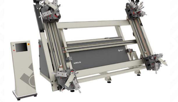
APEX- IVfeatures simultaneous assembling of all 4 corners of the profile by combining the precision of servo positioning and power of hydraulic system to offer quick solutions to users. APEX- IVenables a seamless corner assembling process by minimizing user errors thanks to the two-stage hydraulic pressure system.
