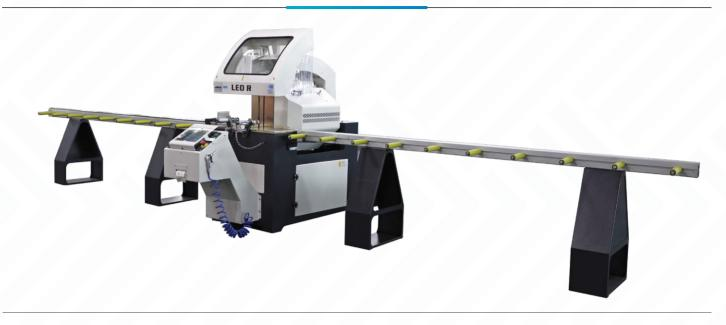
LEO-X, automatic Radial Saw with 2 axis servo controlled and 550 mm saw is ideal for cutting aluminum and PVC profiles with different angles and thickness. LEO-X designed for cutting wider profiles with the servo motion system, automatic positioning at all degrees between 90° and 30° allows for perfect cutting operation. Safety is a topmost priority for LEO-X together with the horizontal clamps and the vertical clamp along with profile protective shield which improve the cutting quality.
