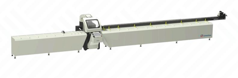
Automatic cutting machine with 550 mm saw blade LEOplus is ideal for cutting aluminum and PVC profiles in various angles and thickness. LEOplus provides rapid and precise process with servo controlled positioning of head at any angles between -22.5° and 45° and servo controlled robotized profile loading gripper. Safety is a topmost priority for LEOplus together with the horizontal and vertical clamps which improve the cutting quality.
