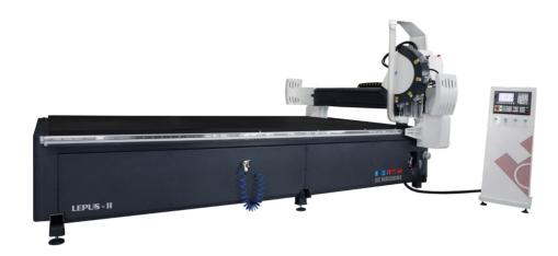
The 3-Axis CNC controlled panel processing machine LEPUS - II is intended for cutting, v-channel opening and similar operations on various composite panels and plates.
