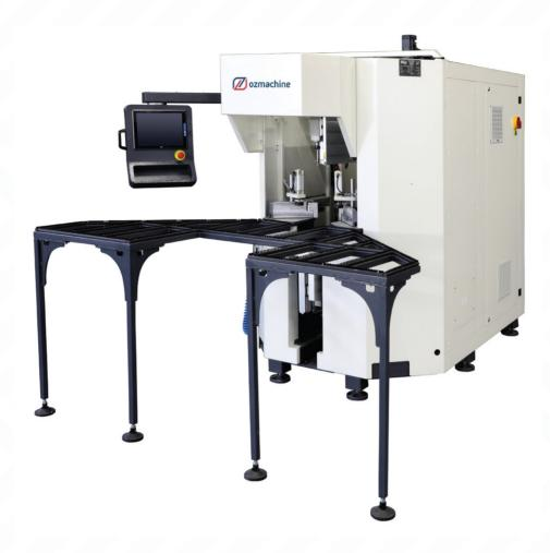
ORBIT - V, the Automatic PVC corner and surface cleaning machine, is developed for cleaning the burrs formed on the plastic profiles after the process of welding. Cleans the lower, upper, inner and outer surfaces of profiles by means of two independent cleaning units. 11 automatic profile cleaning blades provide the users with ease and time saving in burr cleaning process with its 1000 pcs. profile memory capacity and operator adjustable axial speeds.
