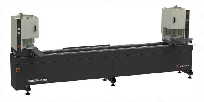
ORION - II SN which is automatic double head zero-normal PVC welding machine, is used for welding processes in various perspectives of plastic profiles. It can weld between 60° and 180° in one head. Through welding time, digital controlled heat and electronic thermostat, it enables to its users to weld between heat values of 0°C - 350°C
