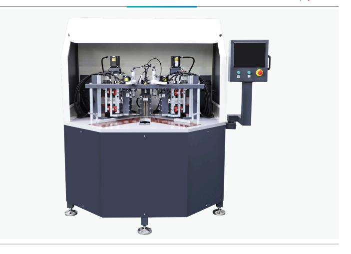
Apex Auto is a corner pressing machine that processes aluminum profiles with completed cutting operations by automatically adjusting the blade settings.
